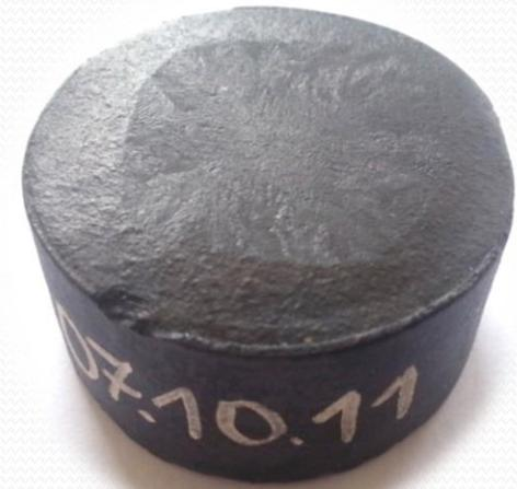
A large, single grain YBaCuO bulk superconductor from [ATZ GmbH](#) (top side machined)
